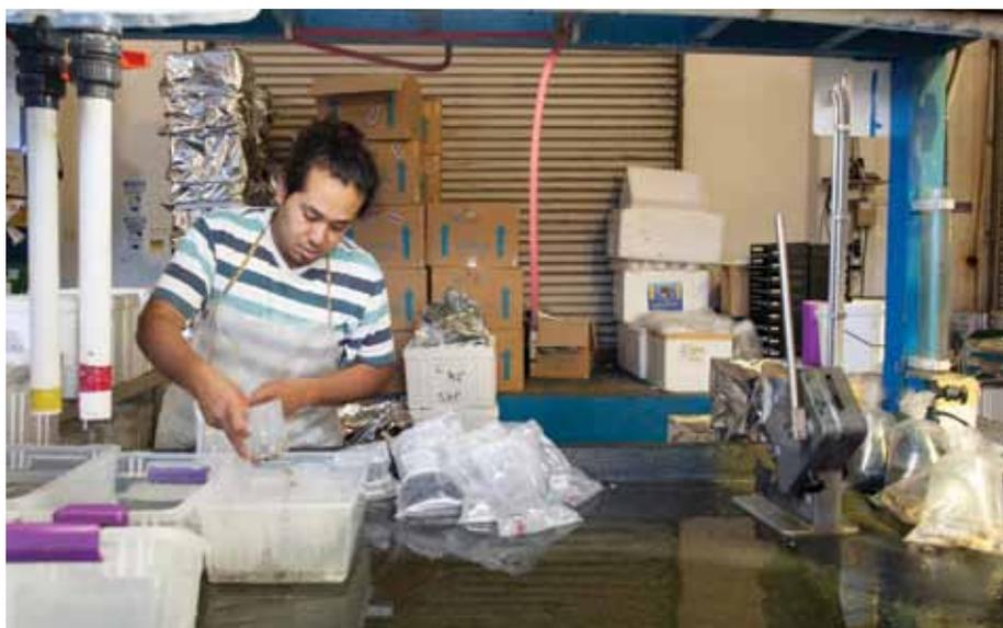
Above: An employee packages fish for shipping, using the pipes on the left to add treated water to each container. The tape on each pipe indicates which is specialized for fish and which for coral.
